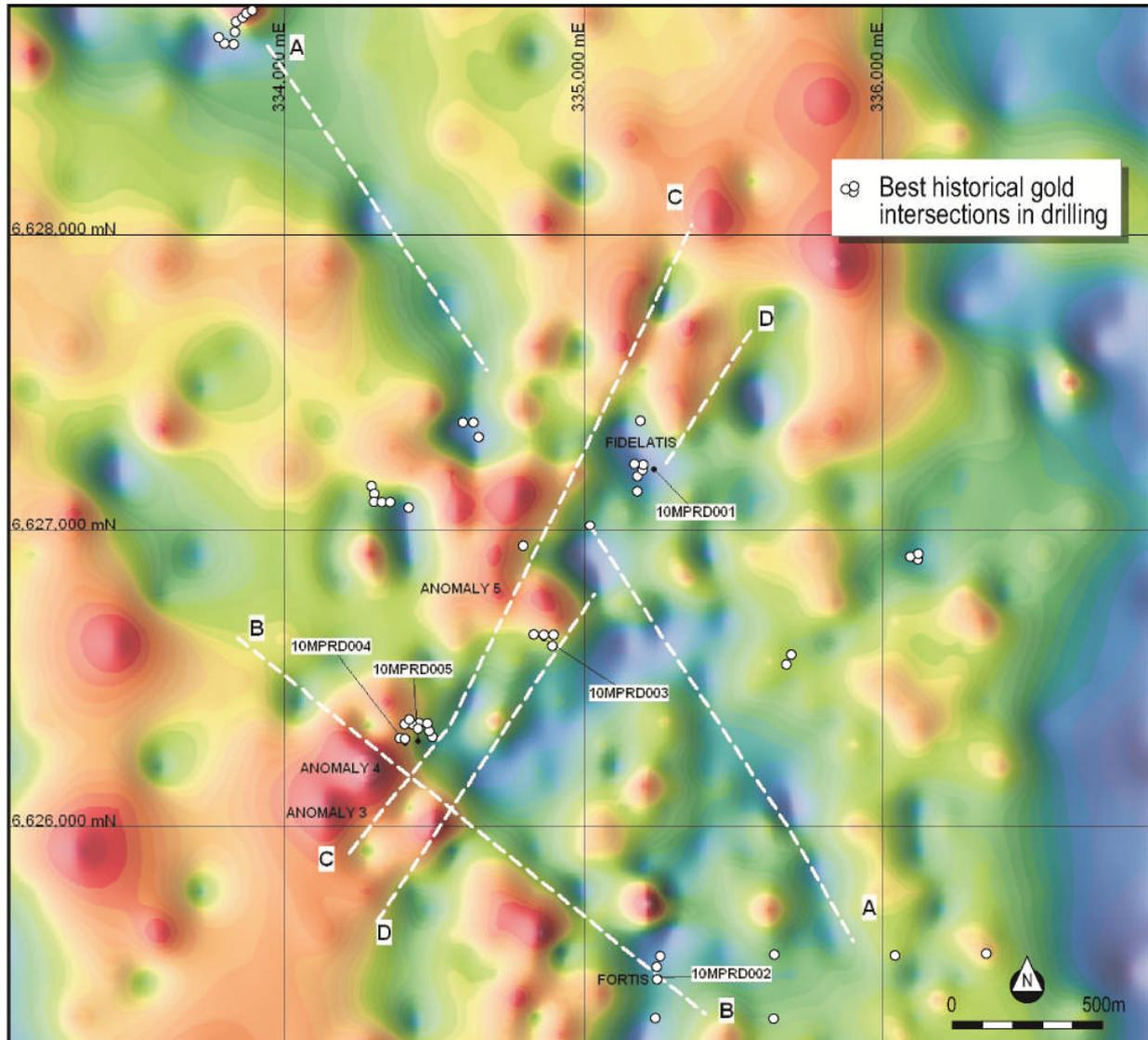
Figure 2. Mt Pleasant gold project - First vertical derivative of Bouguer gravity image/interpretation and drill hole locations.
